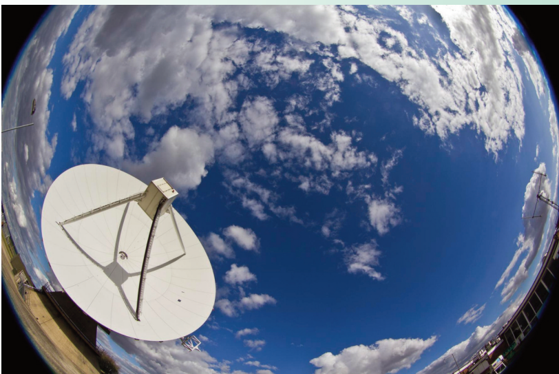
The 25 metre antenna at STFC's Chilbolton Laboratory, which received the first signals from the first satellite of Galileo, the European satellite navigation system.
