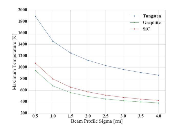
Decreasing the beam width concentrated the energy deposition and increased the maximum temperature.
