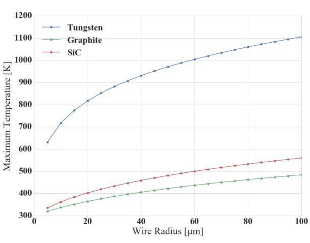
Increasing the wire radius slowed the rate of cooling, increasing the maximum temperature.
