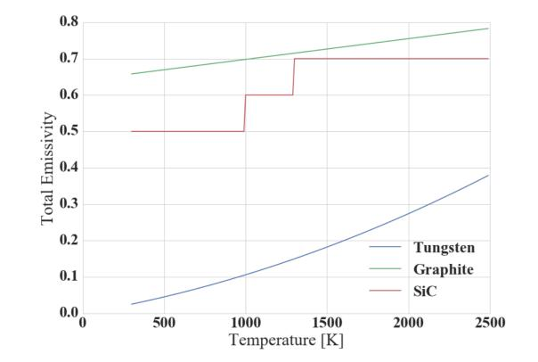
Assumptions were made for temperature dependent total emissivities and specific heat capacities.
