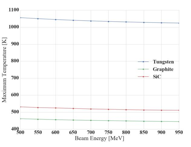
Increasing the beam energy slightly reduces the maximum temperature due to a lower stopping power.
