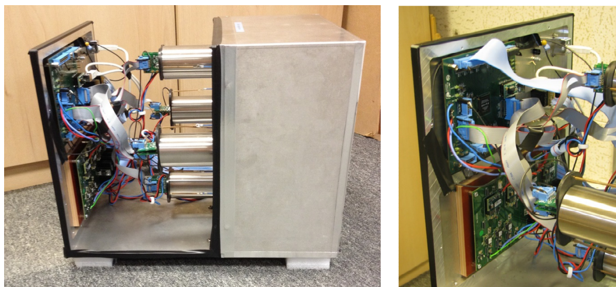
Figure 1. LHS: An ISIS WLS fibre test detector showing the PMT assembly and electronics. RHS: A close up of the detector back plate with the electronics.
